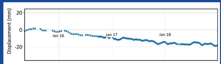
Example of a time series for SatSense data. Each of the blue points corresponds to a new satellite observation of the position of an individual point.
