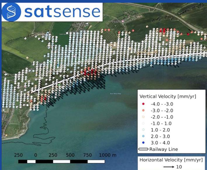
Vertical and horizontal deformation around the Dover-London mainline. Red colours indicate subsidence and blue colours indicate heave.
